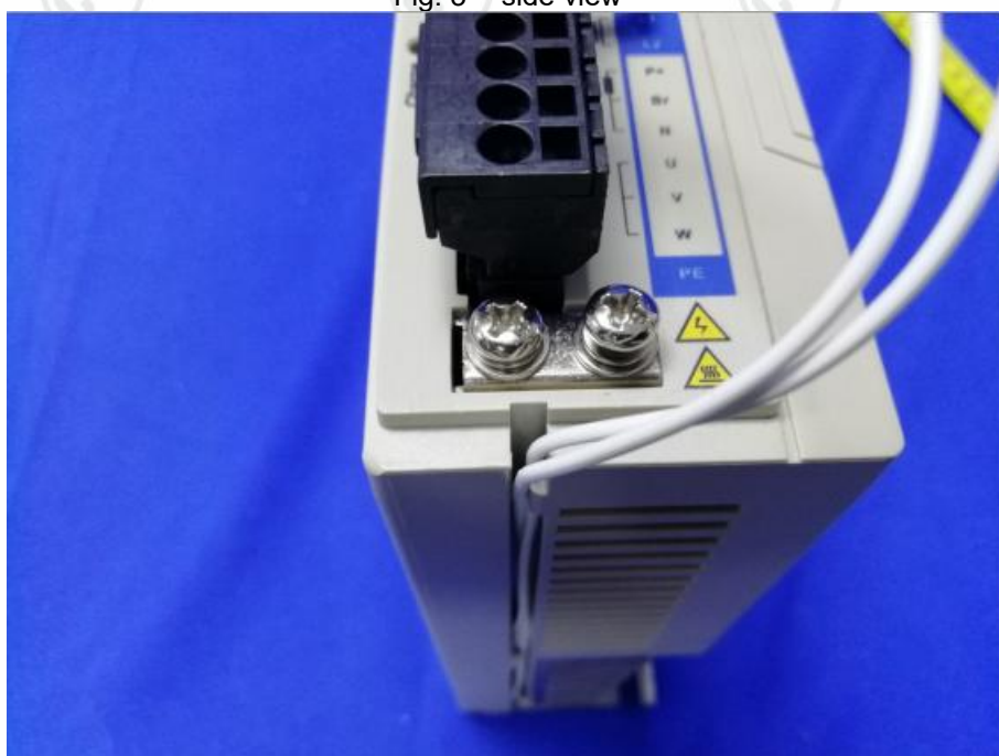
Fig. 4 - Earthing screw
